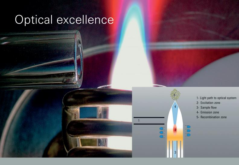
SPECTRO GENESIS utilizes what is likely the industry's best-selling ICP-OES optical system — based on technology common to topline models such as SPECTROGREEN and SPECTRO ARCOS. The main difference: a smaller optical space, which saves gas consumption while still delivering optimized performance for a wide array of routine analyses.
