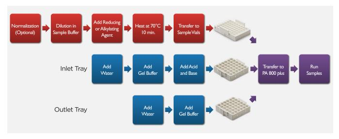
Figure 2. Process Workflow. The Biomek 4000 Workstation is used to automate the preparation of samples (red) and buffer trays (blue). The user transfers the sample tray and buffer trays to the PA 800 plus and runs the samples (purple).
